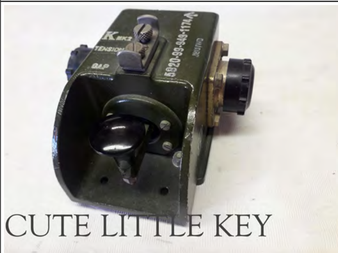
Larkspur Radio Morse Key - Short Arm Type K MK2 (NATO stock no. 5820-99-949-1174)
