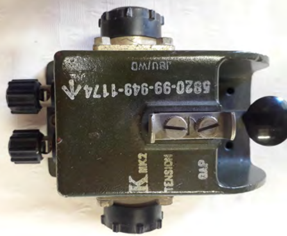
Larkspur Radio Morse Key - Short Arm Type K MK2 (NATO stock no. 5820-99-949-1174)
