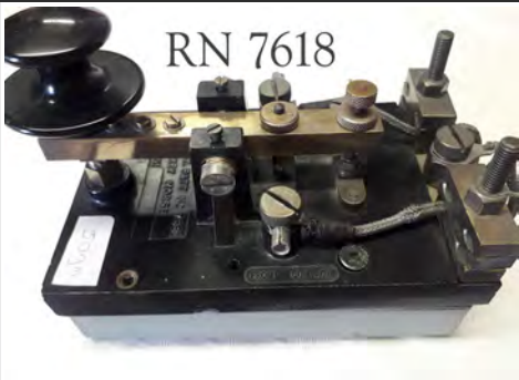
Admiralty key Pattern No. 7681 (1945) with spark quench unit
